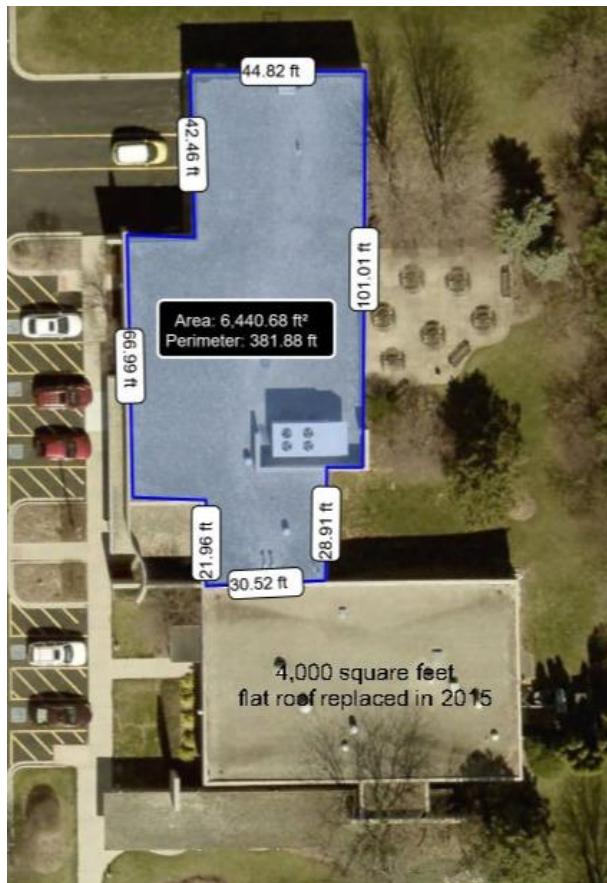
**Description:** The Community Center addition to the Township offices was constructed in 2006. Totaling approximately 6,400 ft<sup>2</sup>, the foot flat roof over this section of the building is aging. The estimated useful life of this flat roof is 20 years. Replacement is being considered in the 2025-2026 fiscal year.
